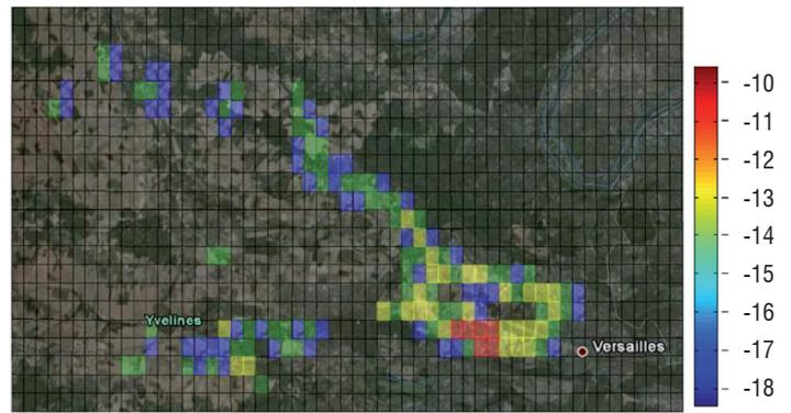
Figure 11 - Map of collision probability estimates with importance splitting. The color scale depends on the logarithm of the probability
