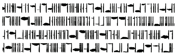
Data sampled by PMS 2DP probe during the P event \perp 6400 \mu\text{m}
