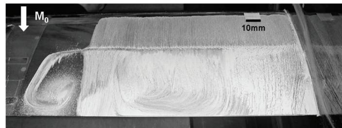
Figure 3 - Oil flow visualization of the upper surface of the wing for  $\alpha = 3.5^\circ$ ,  $M = 0.73$ , viewed from downstream: a) left side, b) right side. The center region of the airfoil is free from oil flow.
