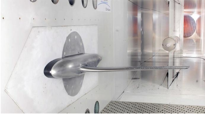
Figure 13 - AVERT model in the S2MA wind tunnel.
