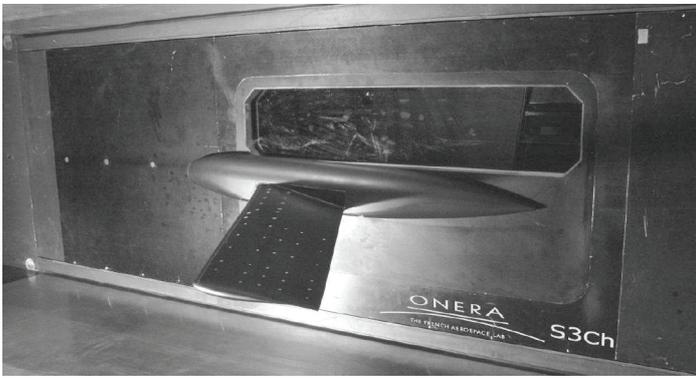
Figure 7 - Experimental set-up in the S3Ch wind tunnel
