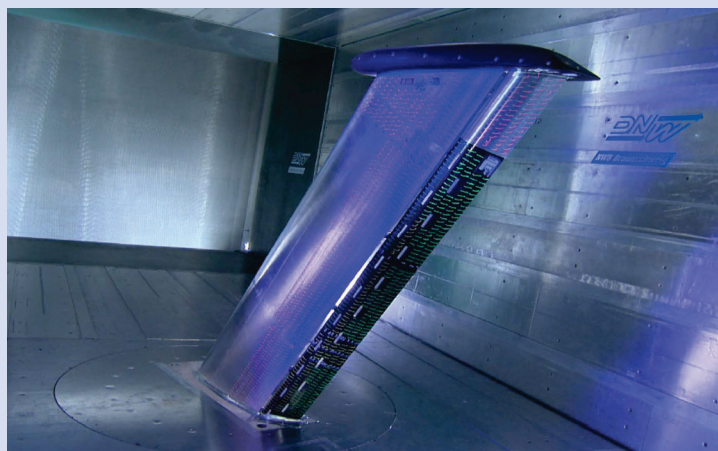
Figure B1- 02 Overview of the mounted swept DLR-F15 model in a DNW-NWB low speed atmospheric tunnel
