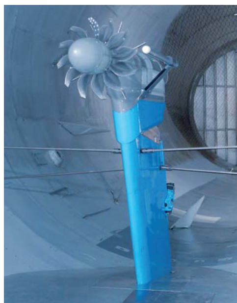
Figure 13 - Snecma's Hera test vehicle mounted in Onera's S1 wind tunnel facility
