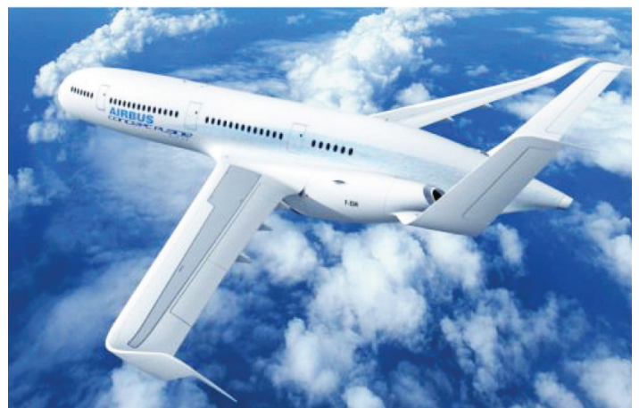
Figure 23 - Airbus views on a futuristic design for 2030 : rearward engines with or without Open Rotors (left) and embedded engines (right).
