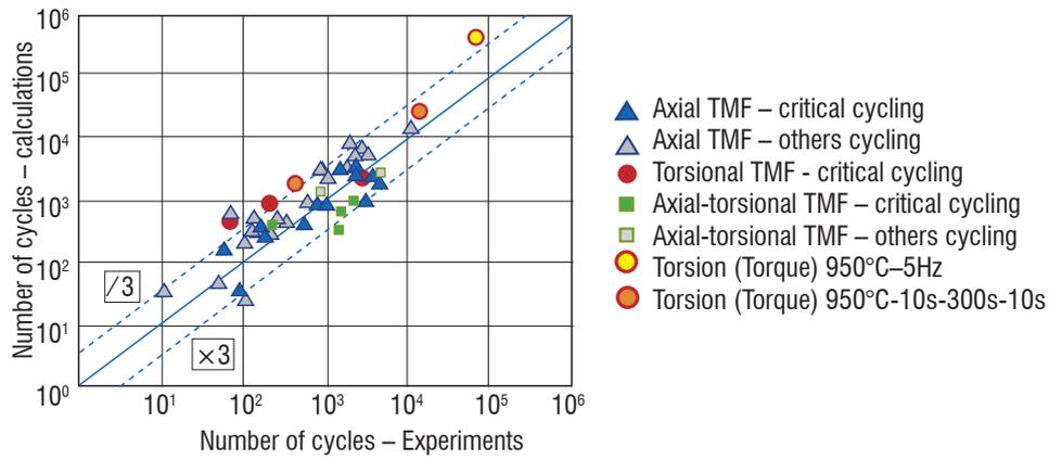
Figure 11 – Lifetime predictions for several anisothermal and multiaxial tests
