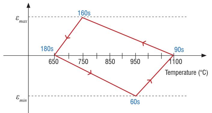
Figure 7 – Thermo-mechanical applied load on cylindrical specimens
