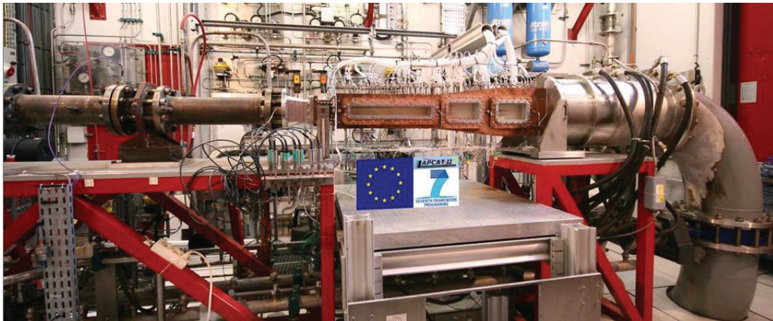
Figure 30 - Lapcat2 combustor installed in the Laerte facility
