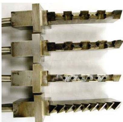
Figure 26 - JAXA strut injector concepts (with streamwise vortices)
