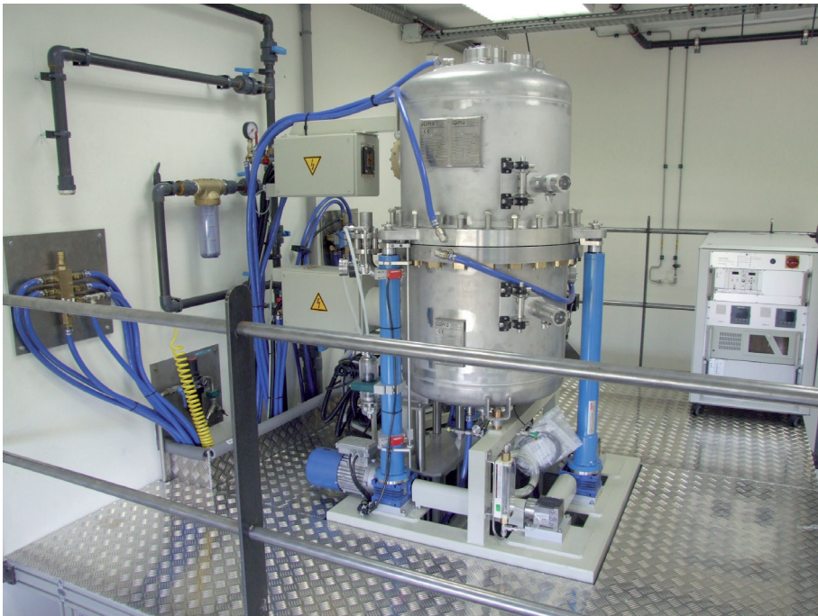
Figure 11 - The Bridgman furnace (a) and an Al 2 O 3 -GdAlO 3 crystal obtained using this furnace (b).
