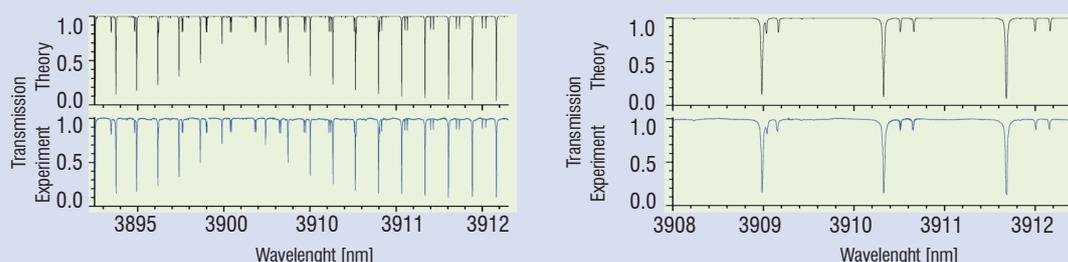
Figure B2 - 06 -  $N_2O$  absorption spectrum recorded at 10 hPa (in blue), the high resolution is illustrated by zooming the 3910 nm region (right side); the most-intense absorption lines are attributed to the  $2\nu_1$  fundamental vibrational band, whereas the doublets of lines are related to the hot vibrational band ( $2\nu_1 + \nu_2 \rightarrow \nu_2$ ).
