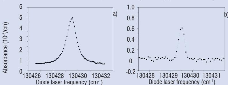
Figure B1-03. Absorption spectra for  $O_2$  in air, recorded during a 280-Hz laser frequency-sweep and a synchronous  $5\text{-}\mu m$  cavity modulation range. (a) At atmospheric pressure, a Lorentzian profile of  $0.095\text{-}cm^{-1}$ -FWHM is superposed to the experimental points. (b) At 20 mbar, a  $0.025\text{-}cm^{-1}$ -FWHM Gaussian profile provides a fit of the plotted points.
