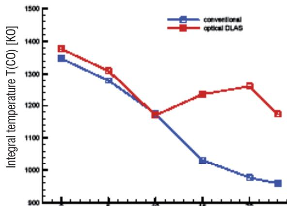
c) Horizontal profile of integral temperatures weighted with the CO concentration at  $x=10$  mm inside the combustor at  $T_3=850$  K and  $T_f=2000$  K
