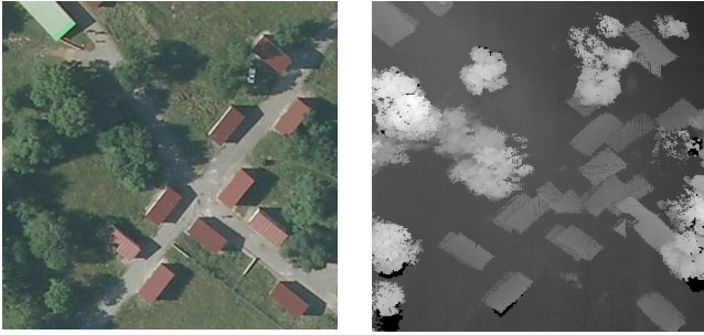
Fig. 2. Comparison of an aerial image (source: IGN) and an altitude map obtained using Lidar data set in the same reference frame from raw navigation measurements. Ghost buildings appear and the scene geometry is distorted, which means a localization drift occurs.
