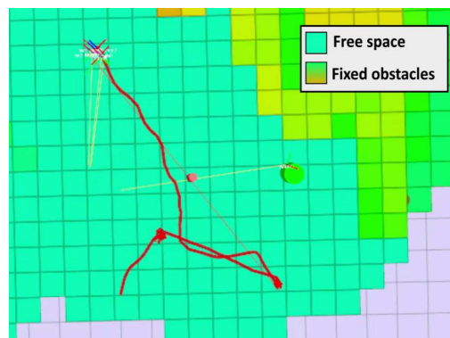
(d) Rviz view (end of mission). Light red line: reference trajectory, Thick red line: MAV trajectory with avoidance maneuver, Green cylinder: object estimated position.
