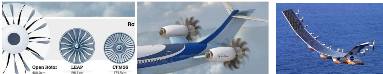
Figure 1 (G) Open Rotor diameter Vs current engines ©Safran; (C) Installed Open Rotor ©Safran; (D) Pathfinder ©NASA.
