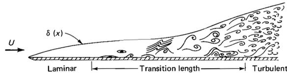
**Figure 2:** Illustration of a transitional region in a flat plate boundary layer [5].
