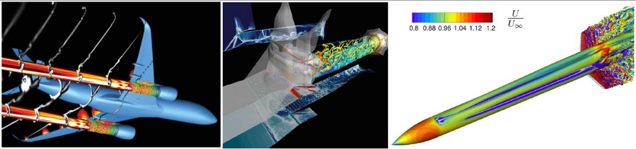
**Figure 1:** Examples of applications of the ZDES technique to complex geometries (wide-body aircraft [3], generic supersonic inlet [7] and generic missile [8]).
