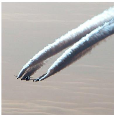
Fig. 1 Condensation trails in the wake of a 4 engine commercial aircraft
