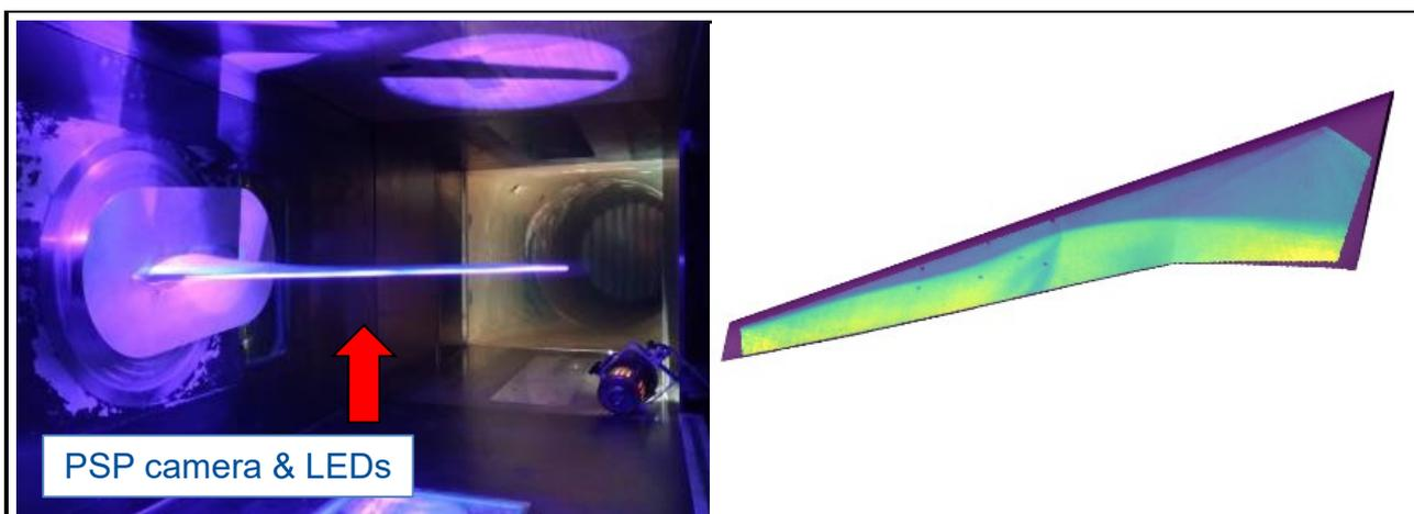
Figure: Pressure field measurements in transonic conditions using unsteady PSP in ONERA S3Ch wind tunnel: photograph of illuminated PSP painted wing in wind tunnel (left), pressure map measured on the suction side by PSP (right)
