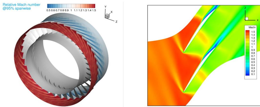
**An example of relative Mach number distribution at 95% blade height for the ROTOR 37 configuration.**
