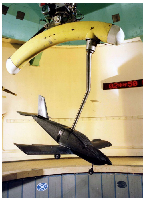
Figure 2 – Scale model of a light aircraft on the vertical wind-tunnel SV4 of ONERA Lille ©Onera
