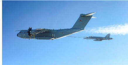
Figure 1 Formation flight. Demonstration of formation flight of A400M aircrafts (left), illustration of the condensation behind the turboprop engine of an A400M during a fighter refueling operation (middle), tests of formation flight in Airbus Fello'fly project (right)
