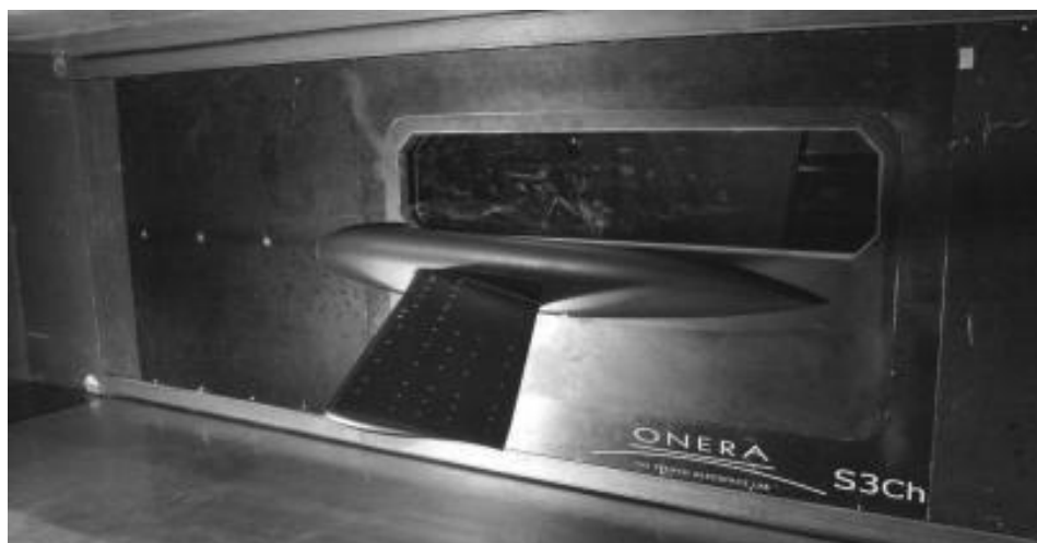
Transonic wind tunnel experiment at ONERA, pressure taps are visible on the wing, from Molton et al., 2013, AIAA Journal 51, 761-772
