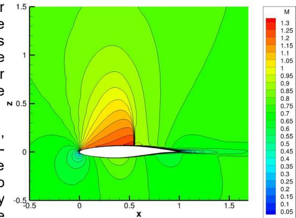
Figure 1: High-order accurate DGSEM simulation of the flow around a RAE2822 airfoil in transonic turbulent flow conditions (color levels: Mach number contours)
