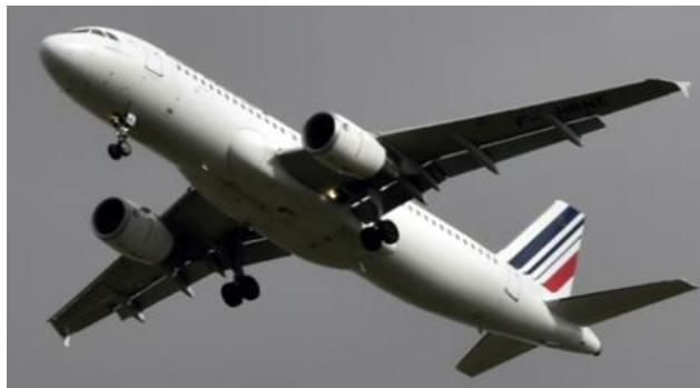
Examples of business jet (top : Falcon F7X) and small-medium range transport aircraft (bottom : A320) at approach, with landing gears and high lift devices deployed
