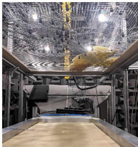
Figure 15: Beamforming array mounted above the Kevlar-walled test section.
