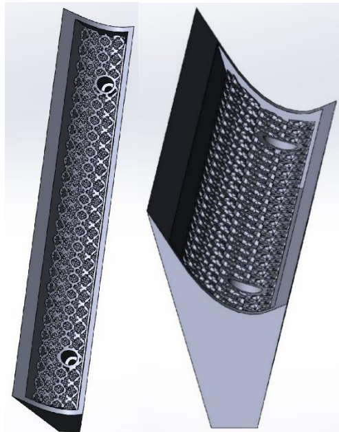
Figure 12: Insert iteration 3. 150 mm long using 6.4 mm diamond-cell lattice. The insert is shown located in a container which will be 3D printed in order to house the insert so that it will not be damaged in shipping.
