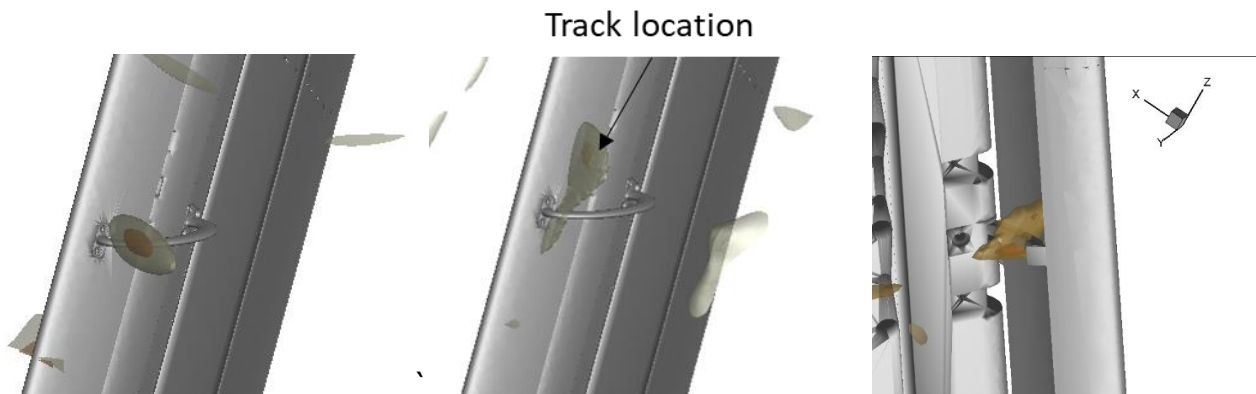
Figure 14 Tomograms for slat track 1; 4kHz (left); 6kHz (centre) and 10kHz (right)
