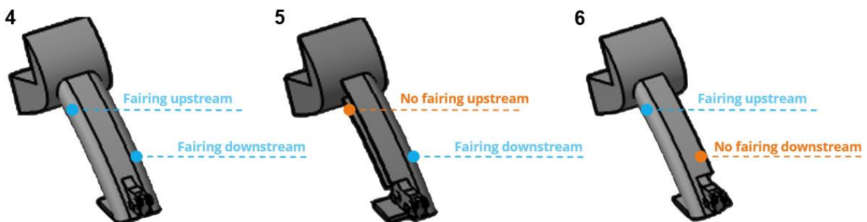
Figure 5: Low-noise slat track designs with upstream and or downstream fairing.
