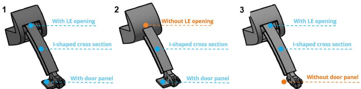
Figure 4: Baseline slat tracks with the differences between them indicated.
