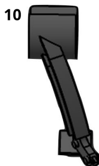
Figure 7: Design of flow-aligned slat track.
