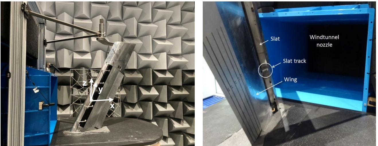
Figure 10: Experimental set-up with the microphone set-up (left) and picture of the set-up (right).
