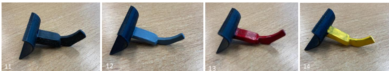
Figure 35: Slat tracks provided by DLR, based on an Airbus design (INTONE project)
