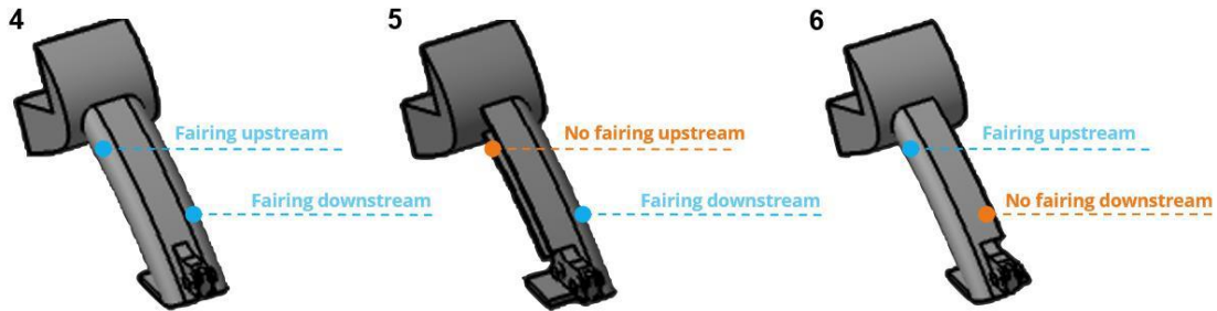
Figure 33: Low-noise slat track designs with upstream and or downstream fairing
