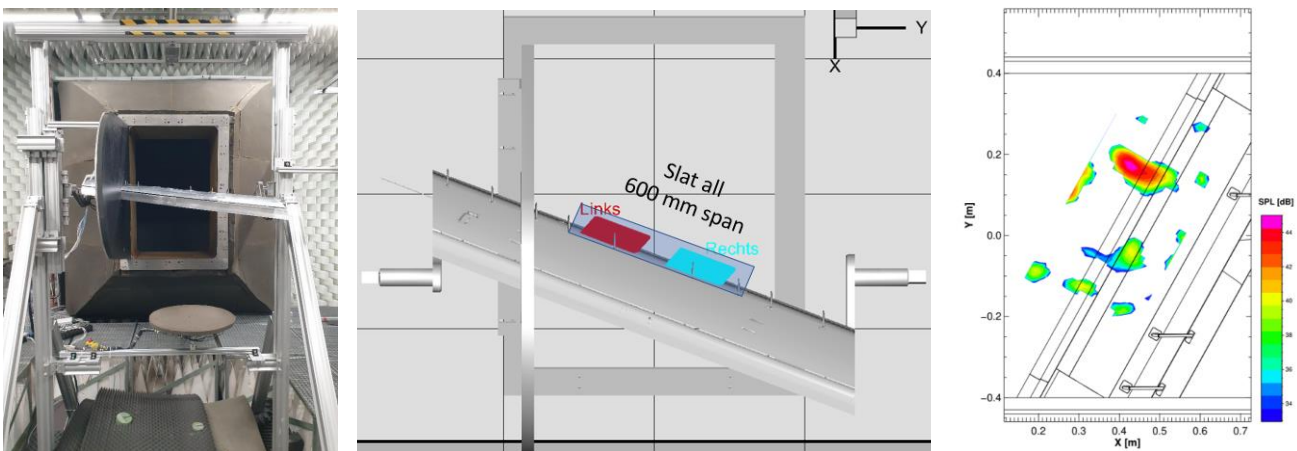
Figure 67: Test-set up of the swept F16 model in AWB for additional tests of porous inserts. Noise map at 8 kHz
