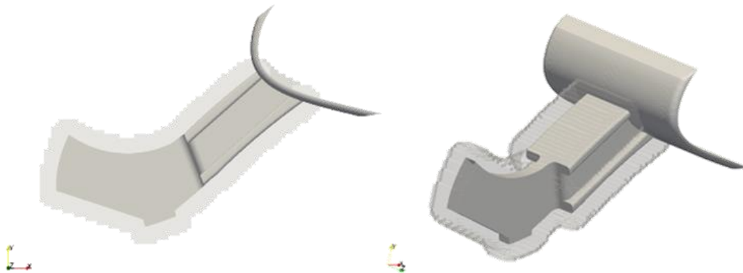
Figure 178: Slat track with a porous glove
