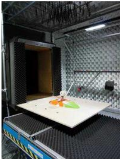
Test set-up in AWB : trailing arm 2-wheel landing gear on a streamlined support
