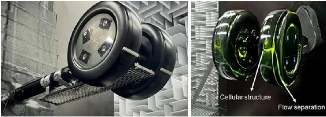
Left : Simplified landing gear equipped with a wiremesh fairing – Right : flow visualization
