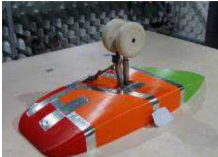
Test set-up in AWB : trailing arm 2-wheel landing gear on a streamlined support
