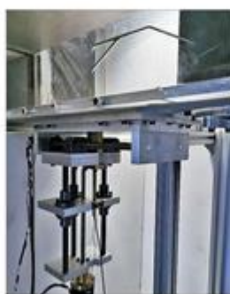
WAABLIEF facility : hotwire set-up (left) - Mean velocity/turbulence intensity intensity traverse profiles at 3 distances downstream the wiremesh sample (right)
