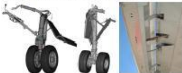
Landing gear architectures (left) and slat actuation and de-icing systems (right) studied in INVENTOR
