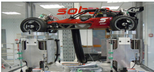
Figure: Car equipped by 4 semi-active suspension dampers.
