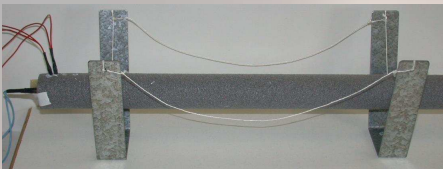
Figure : Thermal aluminium rod heated at one end.
