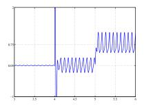
$(\mathcal{L}_2 \text{ gain})$  stability + integral control do not ensure step tracking/rejection for LTV system
