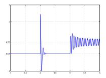
$(\mathcal{L}_2 \text{ gain})$  stability + integral control do not ensure step tracking/rejection for nonlinear system
