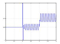
Output y(t) for  $x_0 = 0$ , a step disturbance at 4s and a square reference signal
