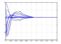
$(\mathcal{L}_2 \text{ gain})$  stability ensures convergence to 0 for different initial conditions
