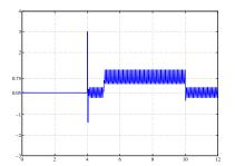
Output y(t) for  $x_0 = 0$ , a step disturbance at 4s and a square reference signal
