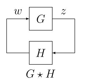
• G: FDLTI  $\begin{cases} \dot{x}(t) = Ax(t) + Bw(t), \\ z(t) = Cx(t) + Dw(t). \\ A \in \mathbb{R}^{n \times n}, B \in \mathbb{R}^{n \times m}, C \in \mathbb{R}^{m \times n}, D \in \mathbb{R}^{m \times m} \end{cases}$ • H: pure delay  $w(t) = z(t - h) (H(s) = Ie^{-sh})$ •  $D \neq 0 \Leftrightarrow$  neutral type positivity?
