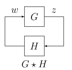
• G: FDLTI  $\begin{cases} \dot{x}(t) = Ax(t) + Bw(t), \\ z(t) = Cx(t) + Dw(t). \\ A \in \mathbb{R}^{n \times n}, B \in \mathbb{R}^{n \times m}, C \in \mathbb{R}^{m \times n}, D \in \mathbb{R}^{m \times m} \end{cases}$ • H: pure delay  $w(t) = z(t - h) (H(s) = Ie^{-sh})$ •  $D \neq 0 \Leftrightarrow$  neutral type
