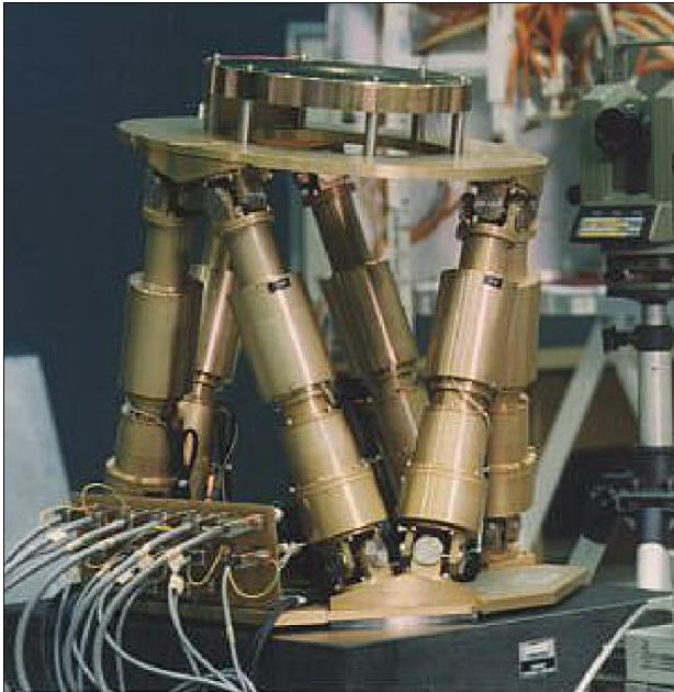
Photo of the Hexapod development model (image credit: Thales Alenia Space-Italy)
