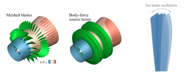
*Left:* Comparison of a turbofan aerodynamic study with conventional 'high-fidelity' and body-force CFD methods. *Right:* Schematic of the oscillation of a blade when subject to an unsteady aerodynamic loading.
