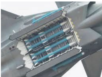
Fig. 1 – (left) Weapon bay of a supersonic fighter as an example of cavity. (middle) Numerical simulation of a cavity and (right) view of the probing of the experimental supersonic Mach 1.5 nozzle in ONERA Meudon wind tunnel.
